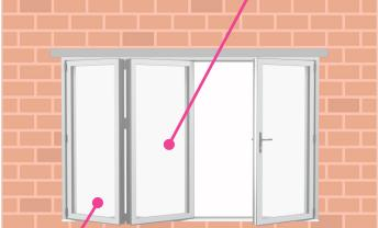
**STEP 12** Replace beading, starting with shortest pieces first and tapping into place with a plastic mallet.
