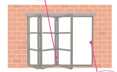
STEP 10 Assess the gaps between the outer frame and sash at the top and bottom, ensuring they are equal. The rolling mechanism can be adjusted to increase or reduce any door gaps - remove the cap and use an allen key to adjust up or down as necessary. Remember to replace the cap after adjusting.
