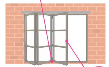
**STEP 14** The latch and hook keeps can be adjusted using an allen key to make any necessary alterations.
