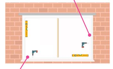
STEP 8 Align the threshold against the cill and fix into place. Use appropriate fixings to secure down through the pre-punched drainage holes into the cill.
