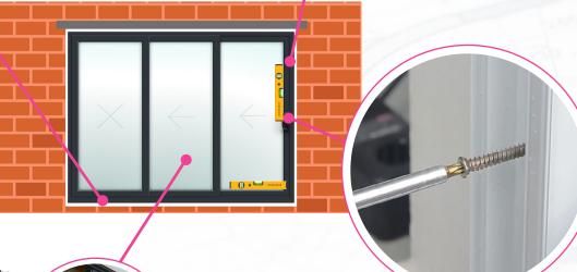
**STEP 7** With the packers in place, fix both outer jambs in place with appropriate fixings.
