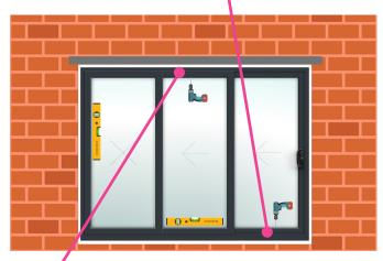
STEP 9 Pack the head parallel to the cill. A timber lat can be used to help ensure it is parallel.
