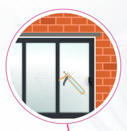
**STEP 17** Ensure all dust & grit is removed from the external surfaces then apply a strip of masking tape to the frame perimeter. Apply a smooth bead of silicone sealant between the frame & brickwork. Remove the masking tape before the sealant sets for a neat, clean finish.
