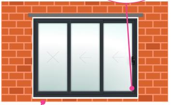
**STEP 20** The rolling mechanism won't work smoothly if there is any debris in the door track, so make sure you clean it properly with a soft brush.
