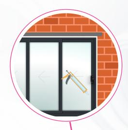
**STEP 18** Ensure all dust & grit is removed from the external surfaces then apply a strip of masking tape to the frame perimeter. Apply a smooth bead of silicone sealant between the frame & brickwork. Remove the masking tape before the sealant sets for a neat, clean finish.
