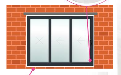
**STEP 21** The rolling mechanism won't work smoothly if there is any debris in the door track, so make sure you clean it properly with a soft brush.
