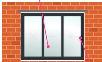
STEP 17 If the sliding door requires adjustment, this is performed at either corner of the bottom sash by adjusting the wheels with a 4mm allen key. These must be adjusted equally so that the door is parallel with the jam.
