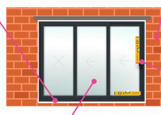
**STEP 7** Lift the sliding door into position in the opening. Hold the door in place temporarily whilst you level it..
