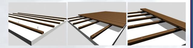
The WPC products' expansion rate is around 0.3% to 0.5% depends on different weather condition in different places, based on this expansion rate, there must always be a gap always between 2 WPC products, as follows:
