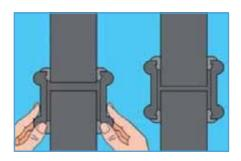
6. . When cut ting into an existing cast iron soil system a slip socket with ears should be used. This has no central register and allows the socket to be slipped onto the existing pipe up to the second gasket before placing the new fitting in position.
