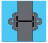
7. Slide the eared socket into the correct position where the respective gaskets make a seal on the pipe/fitting on either side of the joint.
