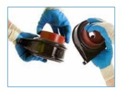
1. To aid insert ion of the components, immediately prior to assembling the joint, pre- relaxation of the rubber gasket is recommended. Apply a small amount of lubricant to the rubber gasket and inser t the relaxing tool into the joint. Slide the relaxing tool up and down over the gasket sealing face three or four times. The gasket will now be temporarily sof ter and enable easier assembly of the soil s tack joint. Caution: Do not over insert the relaxing tool past the rubber gasket.
