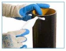
2. Apply a small amount of lubricant to the rubber gaskets at both ends of the push fit socket. This is necessary to ensure the insertion of pipes and fittings into the socket.
