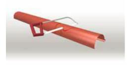
Note: Never use an angle grinder to cut the gutter as it will burn the polymer layer and could possibly lead to corrosion – always use a hacksaw.
