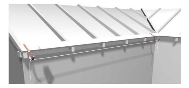
All other brackets should be fixed at 800mm centres. In areas of potentially heavy snowfall we suggest that 600mm centres are used. Brackets are screwed to the fascia board using 25mm BZP screws. Fascia brackets should be installed within 150mm of any angle or running outlet to ensure the fitting is properly supported.
