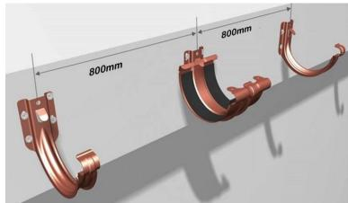
In areas of potentially heavy snowfall you should reduce the fixing centres to 600mm
